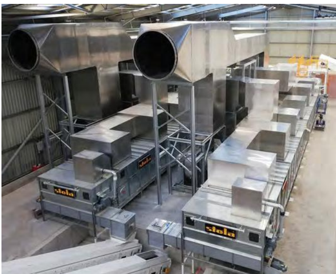
Nawrocki Pelleting, Great Britain: Type: 2 x BTL 1/3000-20 – Product: SRF Dryer output capacity: 4.5 tph from 20 – 10% MC.
