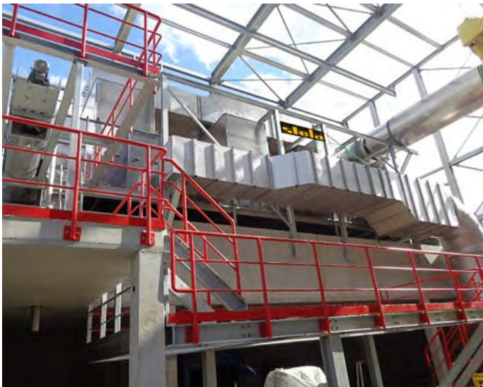
Undisclosed German cement plant: Type: BTL 1/3000-14 – Product: RDF Dryer output capacity: 8.9 tph from 15 – 5% MC.
